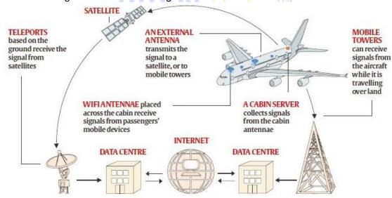
On the ground data is routed through standard channels. The response then travels the process in reverse, explaining the typically slow Internet speeds typical on aircraft
